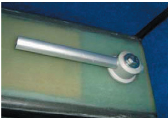
Spar pin - installed
