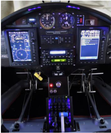
Figure 3 Glare-shield and breakers UV-LED lights
