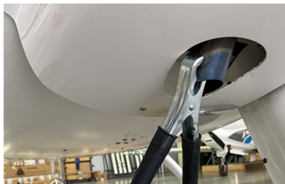
Grounding wire connected to the exhaust
