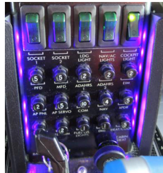
Figure 6 Circuit breakers UV-LED lights
