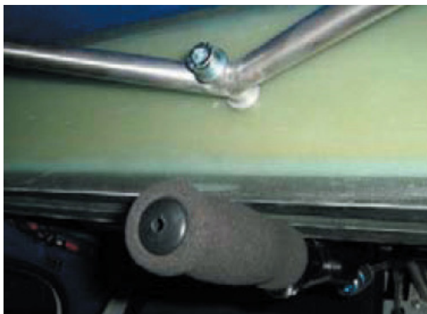
Central wing spar bolt - installed
