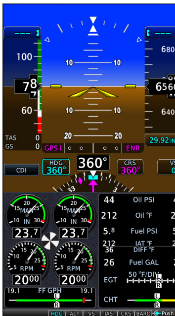
Figure 7-1 Twin Piston Display Backup
