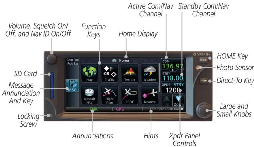
Figure 2 - GTN 635/650 Control and Display Layout
