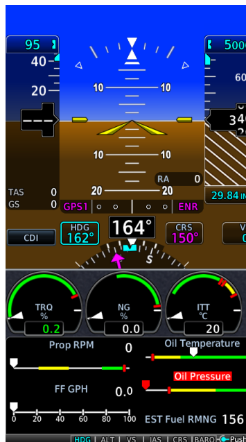
Figure 7-2 Single Engine Turboprop Display Backup
