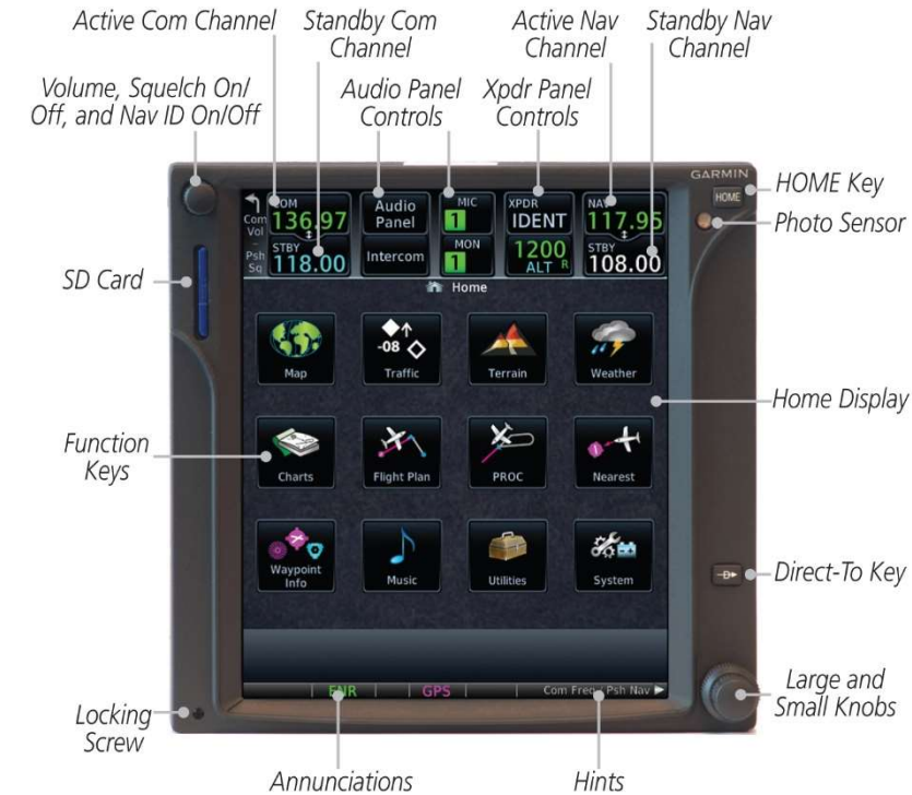
Figure 1 - GTN 750 Control and Display Layout
